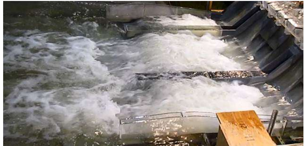
Spillway PMF discharge in General Model
