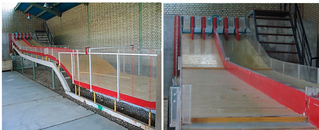
Figure 15. The 1/64 scale model of the Karkheh Dam's spillway.
